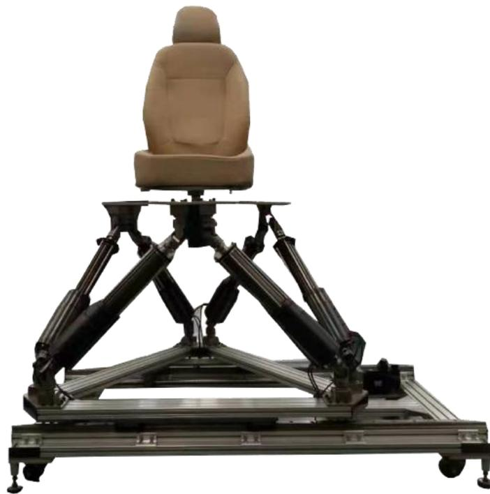
KRD61 series 6-DOF simulation table is a closed-loop servo simulation platform consisting of six servo actuators and six sets of dedicated hinges connected at the top and bottom platforms respectively. By virtue of the telescopic movement of the six actuators, the upper platform moves in six degrees of freedom (X, Y, Z,  $\alpha$ ,  $\beta$ ,  $\gamma$ ), so various space motion attitudes can be simulated.
